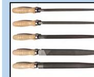
**Files** – used to remove small amounts of material from a workpiece usually to smooth a surface. Commonly used in woodworking and metalworking,
