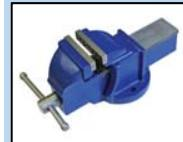
**Engineer's vice** – Used for holding work whilst sawing + filing materials. It sits above the workbench and in the school workshops it is clamped into a woodworking vice
