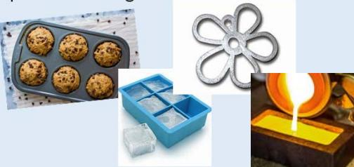
The **mould** is the negative shape. It is the starting point of the moulding and casting process. The liquid is then poured into the mould creating the **cast** which is the positive shape.
